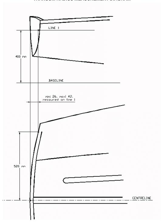
8.8 Section templates 2, 5 and 8 shall be applied as shown on the measurement diagram. The top of deck at the sheerline shall not be more than 10mm above or below the sheer marks on the template. The templates shall touch the rubbing strips or clear. Below the points marked on the templates they shall touch the hull or clear by not more than 16mm, and the total difference between the greatest and least clearances shall not exceed 12mm.
