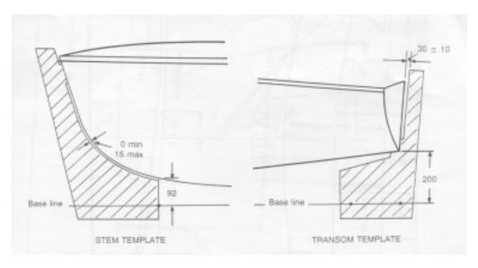
8.7 The transom template shall be applied as shown on the measurement diagram above. The distance between transom and template shall be 20 mm minimum and 40 mm maximum.
